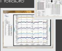
The system components are configured and alarm thresholds set via TMS Manager, a Windows application. Logged data can also be downloaded or viewed in real time.
