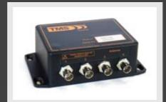
Connecting the TMS Operator Interface displays tire pressure and alerts when any alarm condition is activated. It is configurable for up to 6 wheels, and the unit has a real-time log feature.
